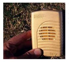
Figure 5: T82 Carbon monoxide monitor
